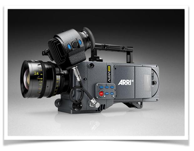
65mm digital cinema camera, ARRI A3X CMOS Sensor Aperture equivalent to 5-perf 65mm film, 6560 x 3102 Resolution 54.12 x 25.58 mm Sensor size (active image area) Sensor image diagonal: 59.87 mm ARRI XPL Mount (64 mm diameter) No over speed at launch, but the camera architecture is capable of supporting a sustained recording data rate over 2 Gigabytes (not bits) per second. current data rate is 860 Megabytes (not bits) per second. so some over crank should be possible in the future.
